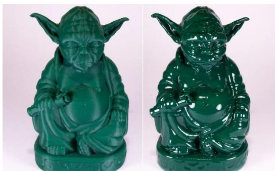
Figure 3.2. ABS – after printing and smoothing [4]
