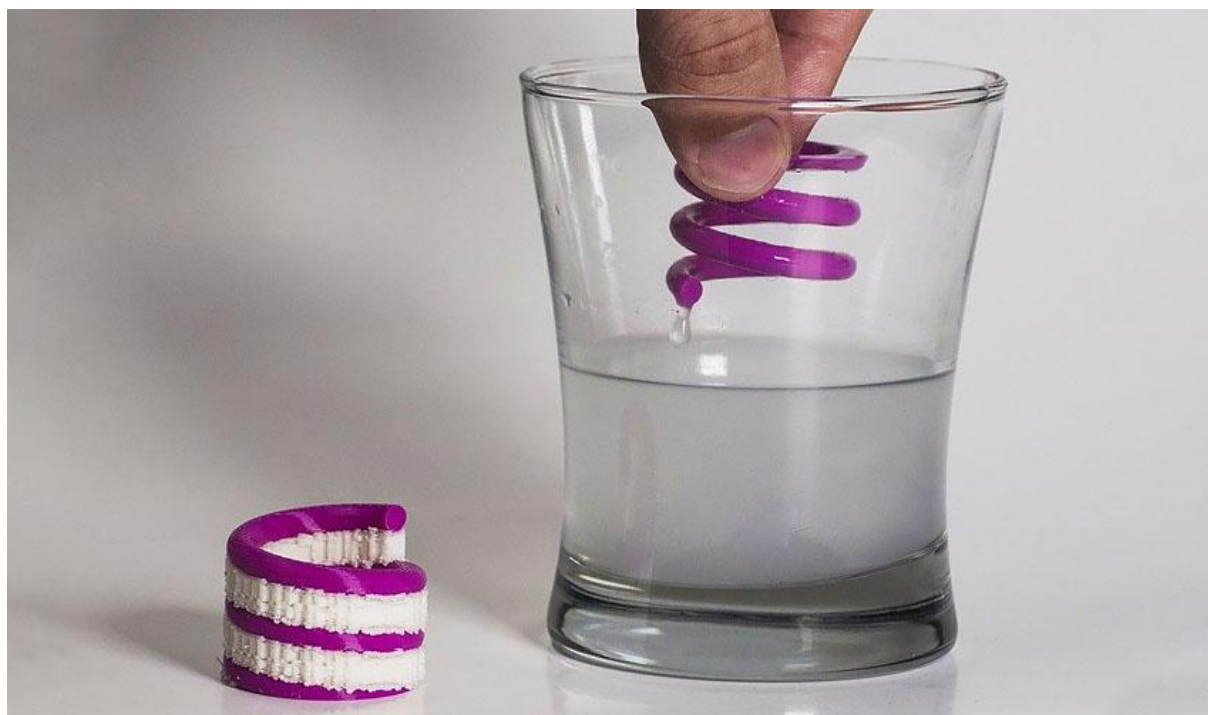
Fig. 3.6 3D print with hips support dissolved in water [10]
