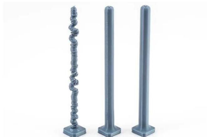
Figure 2.4 First element from the left show overheating problem [5]
