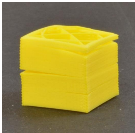
Figure 2.6 Layer separation and splitting [7]
