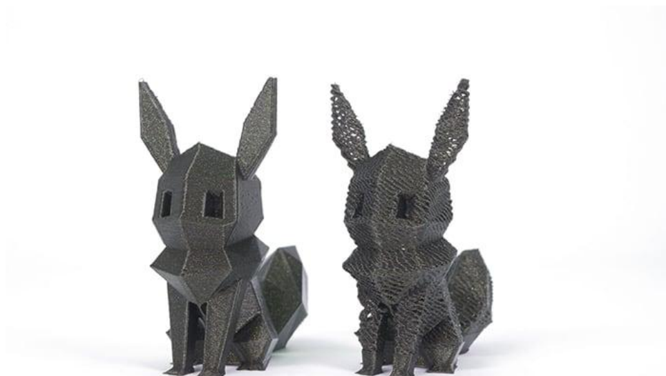
Figure 2.1 Comparison - correct extrusion on the left and under-extrusion on the right [2]
